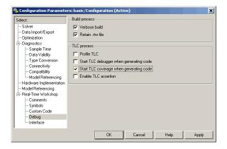
When you initiate TLC coverage, the Target Language Compiler produces a .log file for every target file (\*.tlc) used. These .log files are placed in project directory created for the model. Each .log file contains usage (count) information regarding how many times it encounters each line during execution. Each line begins with the number of times it is encountered, followed by a colon, followed by the code.
