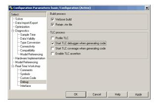
Selecting Start TLC debugger when generating code is equivalent to adding -dc to the RTW System target file field in the Real-Time Workshop pane of the Configuration Parameters dialog box.
