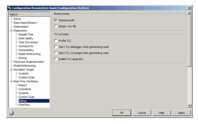
The **Start TLC debugger when generating code** check box lets you activate the TLC debugger. This is covered in more detail in Chapter 7, "Debugging TLC Files".
