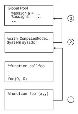
**File Scope.** File scopes are searched before the global scope, as shown in the following diagram.
