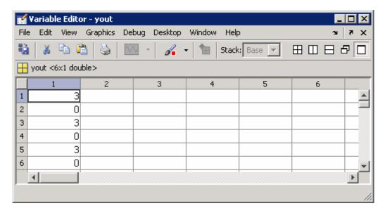
Column 1 contains discrete pulse output for six time steps (3s and 0s), collected at port out1.
